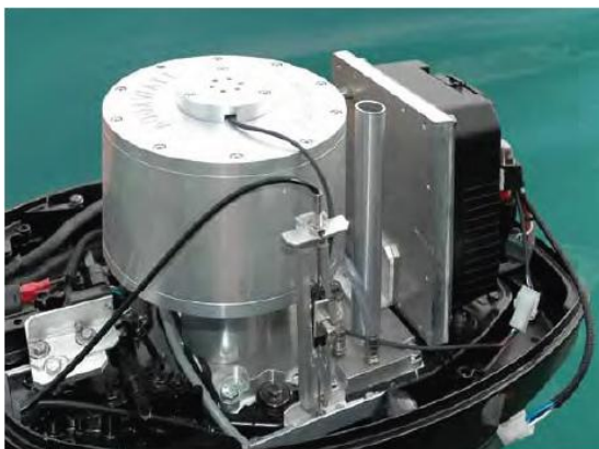
Open powerhead showing motor and controller
