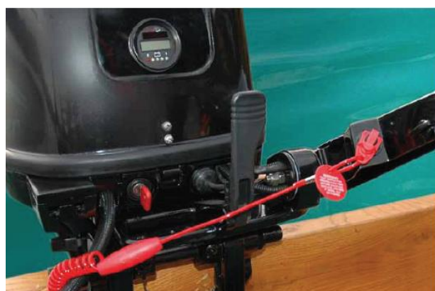
Security switch, tiller and built in control panel
