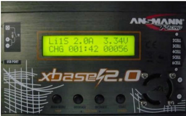
The electronic chargers usually show the charging voltage, not the voltage of the cell. Therefore you have to measure the cell voltage with a separate volt meter. After the charging process, you have to disconnect the cell for a few hours and recharge if the voltage drops.
